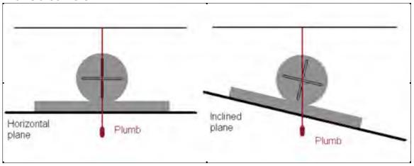
'Sparavigna says that if the straight bar part of the object were laid on a slope, a plumb line would revealed its inclination on the circular dial (as illustrated in this graphic).
